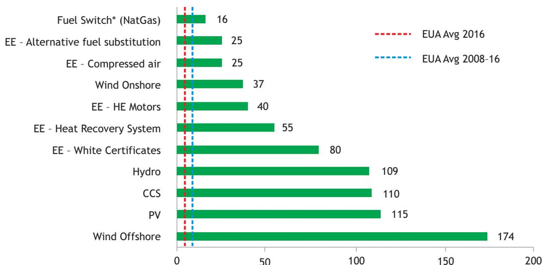
Marginal Abatement cost are calculated on the basis of an average EU wholesale price for electricity of 40 €/MWh (130 €/MWh retail price for industries) and an average EU carbon emission factor of fossil generation of 700 gCO<sub>2</sub>/kWh
